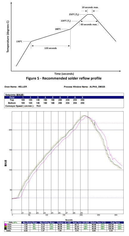
Figure 6 - Example solder reflow profile (AMW006-E03 evaluation board)
