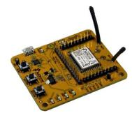
Figure 9 - AMW006-E03 eval board with wire antennas
